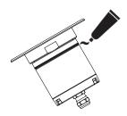
3 Oceano products are tested and guaranteed IP66 / IP68. However, it is recommended to connect the product with gel moulds or IP68 connectors to avoid problems with the electrical sy stem.
