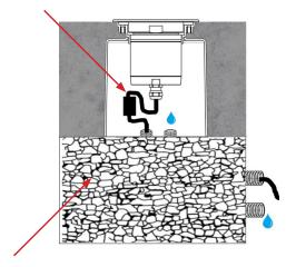
The bottom of the formwork must be in contact with draining material in order not to allow water to stagnate for long periods and to facilitate drainage through pipes.
