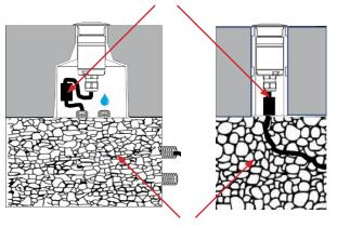
The bottom of the formwork must be in contact with draining material in order not to allow water to stagnate for long periods and to facilitate drainage through pipes.
