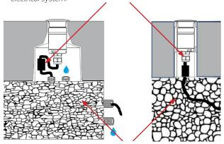
The bottom of the formwork must be in contact with draining material in order not to allow water to stagnate for long periods and to facilitate drainage through pipes..
