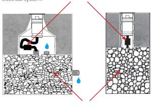
The bottom of the formwork must be in contact with draining material in order not to allow water to stagnate for long periods and to facilitate drainage through pipes.
