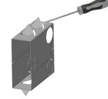
Use a bolt cutter to open one of the two holes for the corrugated pipe.
